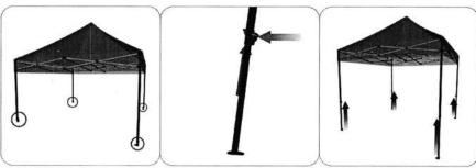
The frame will have four slide locks, one for each corner. When the tent scissor frame is fully extended; make sure the prong of the slide lock snaps into the tube locator hole. Press the lever on the slide lock to disengage the prong from the tube allowing to slide the lock up or down during assembly.
